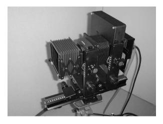
Figure 1. Developed multi-band camera
