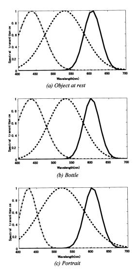
Figure 7. Optimized spectral transmittance of RGB filter in three different objects
