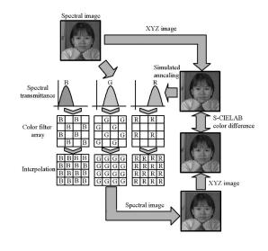
Figure 6. Schematic diagram of filter optimization process
